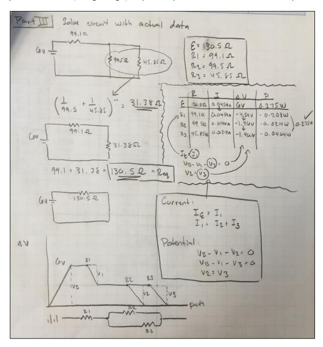
Figure: Multiple Representations of a Circuit
